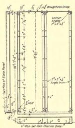
Fig. 209.—Angle-iron frame for switchboard.\*
